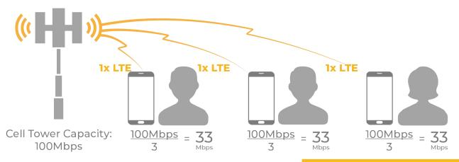
In this example, three users with three LTE-enabled devices connect to a cell tower. Each gets 33Mbps, which is a third of the available bandwidth at the tower.
