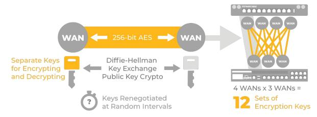
Once the bandwidth bonded SpeedFusion tunnel is formed, sessions are broken down and the resulting packets are sent separately across as available WAN-to-WAN connections. Because each WAN-to-WAN connection is encrypted separately, potential hackers would need to obtain the key to every WAN-to-WAN connection before they stand a chance of accessing the data contained within. This makes SpeedFusion SD-WAN technology virtually impervious to man-in-the-middle attacks.
