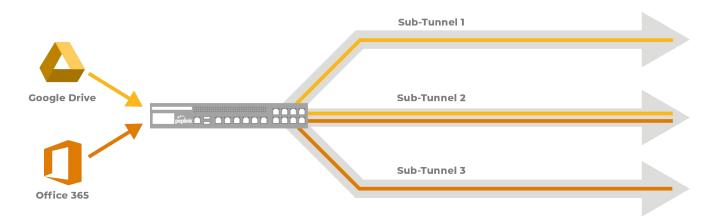
This is achieved through user defined sub-tunnels. Within a SpeedFusion connection, you can define up to five sub-tunnels. Within each sub-tunnel, you can specify which WAN connections to use, set bandwidth limits, as well as configure WAN smoothing and FEC. Once you have defined these tunnels, you can then use outbound policy to steer traffic based on protocol (TCP vs UDP), Port, and Application.
