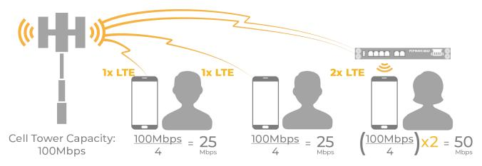
In this example, the third user is using a Pepwave MAX device and has installed an additional LTE data SIM. There are now three devices with four LTE connections connected to the cell tower.
