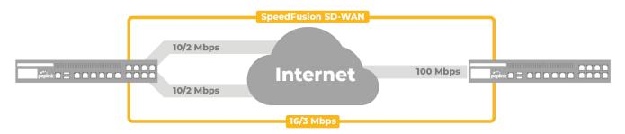
Accounting for SpeedFusion bandwidth overhead and assuming the traffic passing across the links is similar to the IMIX standard mentioned previously, we can calculate available real-world bandwidth at the remote site:
