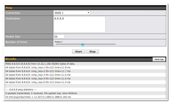
A system administrator can use the ping utility to manually check the connectivity of a particular LAN/WAN connection.
