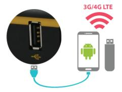
For increased WAN diversity, plug in a USB LTE modem as a backup. Peplink routers are compatible with over <u>250 modem</u> <u>types</u>.
