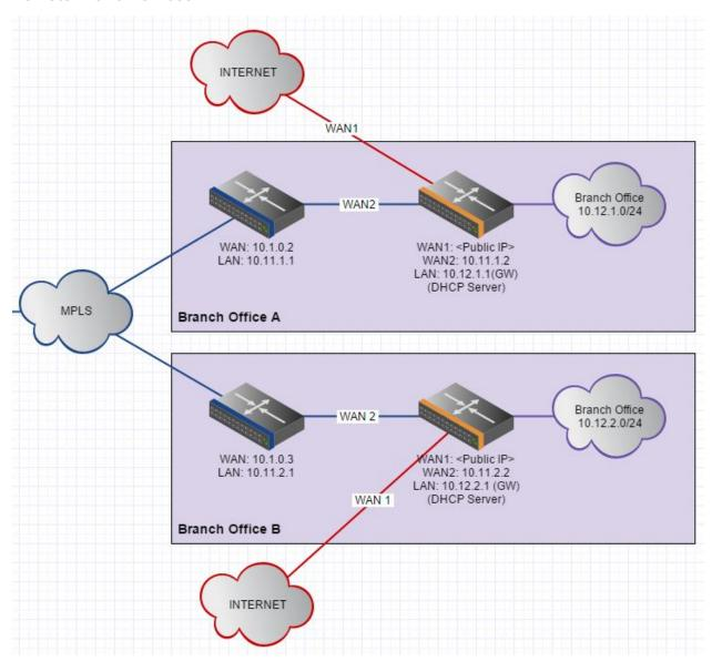
In the remote branch offices a new Peplink Balance router is added to act as the gateway device for the local network and the branch office subnet is changed to be in the 10.**12**.x.0/24 range.
