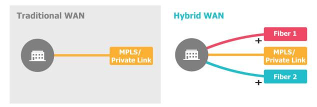
The end result is a Wide Area Network made up of multiple connections between each location that can be actively used at the same time to improve connection reliability and aggregate bandwidth.
