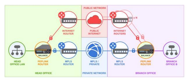
In this example, the head office network now has three routers. A Peplink Balance device has been added to act as the default gateway for the network. This has the public Internet access router and the private WAN access router connected to its WAN ports.
