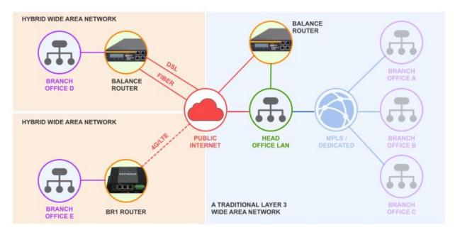
With the simple addition of a couple of static routes on the private WAN and public Internet access routers, the new branch office locations added in this way can communicate securely with both the head office LAN devices as well as the remote branch locations on the traditional WAN.
